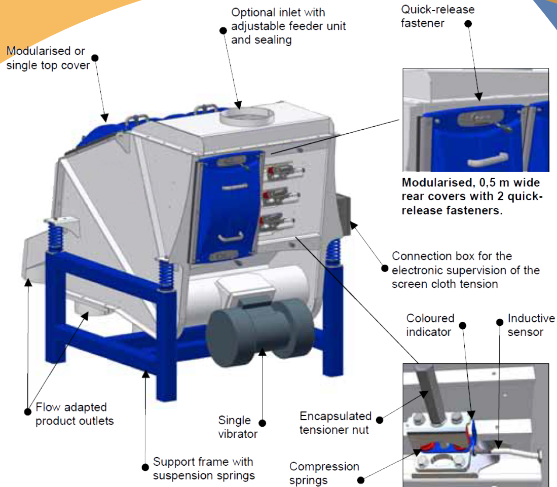
Screen cloth tensioning with electronic remote supervision
