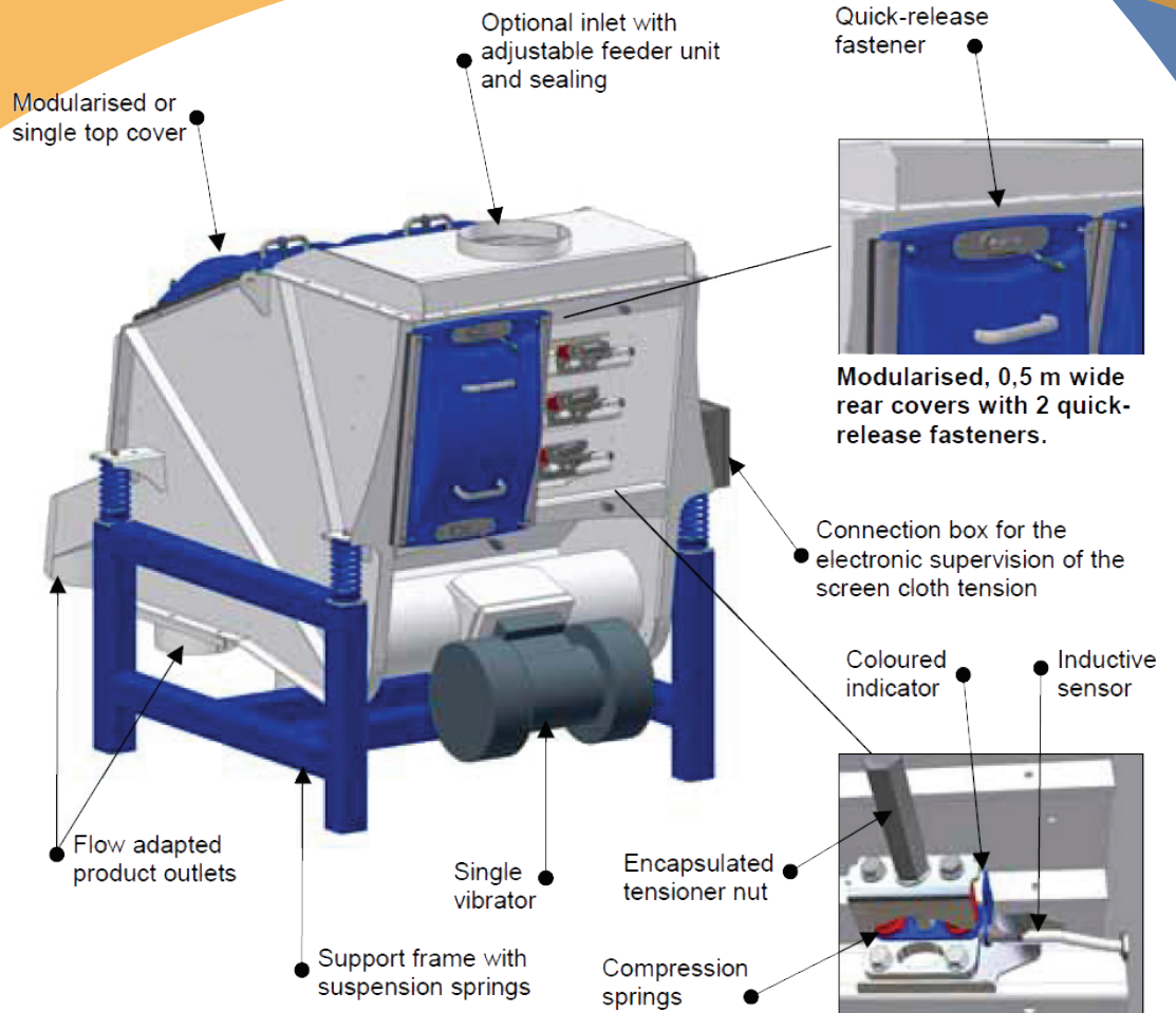
Screen cloth tensioning with electronic remote supervision
