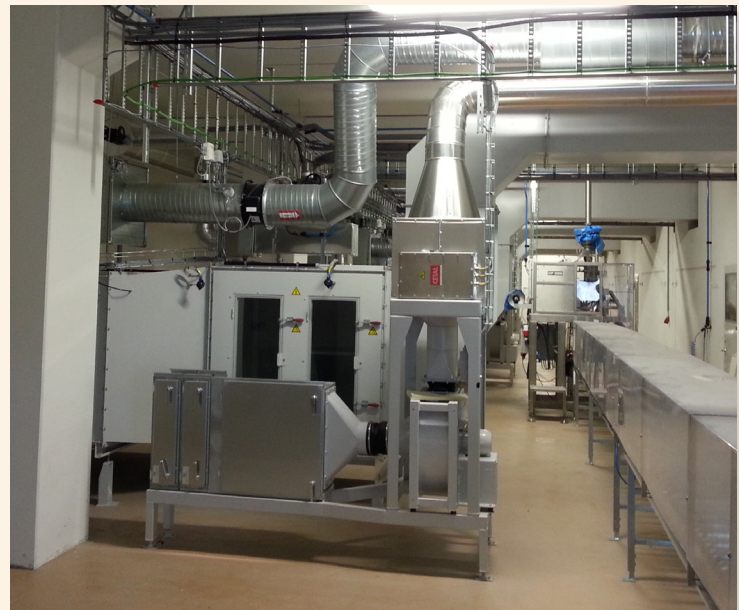
System : heating unit with filter for pellet mill, LT conditioner and steam mixer
